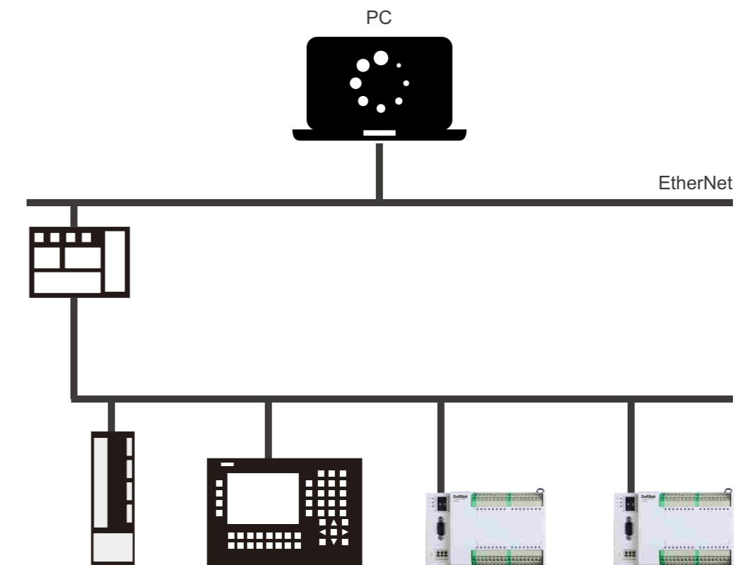
Modbus is one of the industrial field bus protocols. ModBus network has only one host. All communications issued by the host, this protocol supports traditional RS-232, RS-422, RS-485 and Ethernet devices. There are two kinds of transmission modes to choose from the ModBus system, a model to ASCII, another mode is RTU, the network can support as many as 247 remote slave controllers, but the actual number of slaves depend on the used communication equipment.
