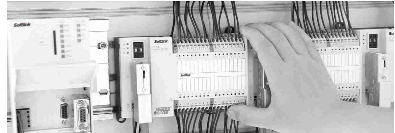
It is a great impact on modern automation system that more and more real-time Fieldbus technology, and centralized control equipment are replaced by distributed intelligent devices. Signal attenuation often occurs during long-distance data transmission, long distance transmission also causing signal interference. Distributed I/O system is a good solution for long distance communication.
